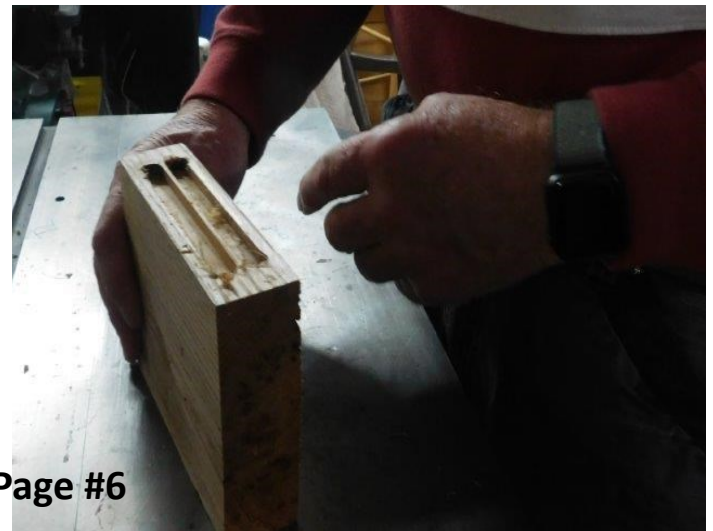
Rolf Dries demonstrated hidden wall fasteners to hang a shelf and conceal the hanging method.
