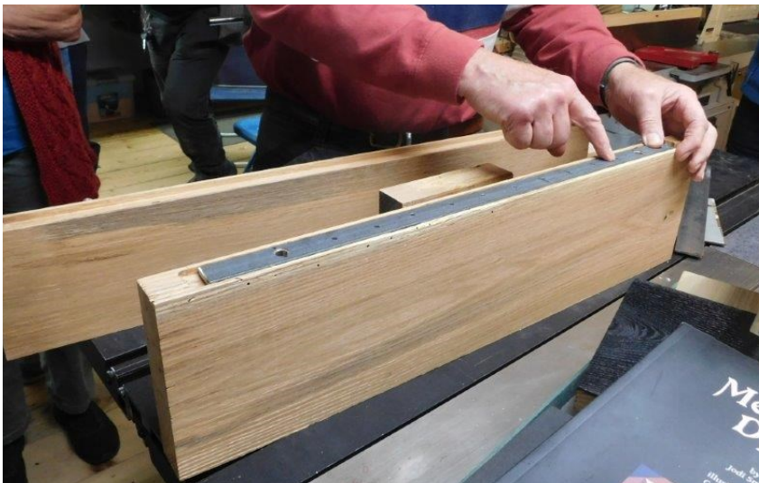
Rolf Dries demonstrated hidden wall fasteners to hang a shelf and conceal the hanging method.
