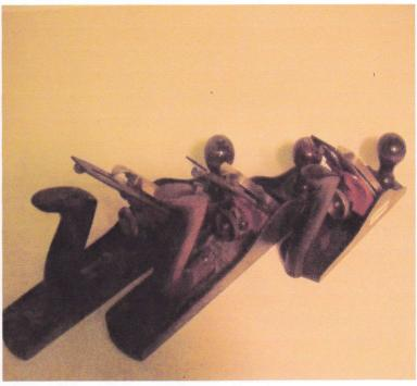
Both photos, front & rear view: Three MILLER FALLS bench planes in good to very good condition. Blades have a lot of sharpening length remaining. These planes have double action clamps. The two planes on left are #14's (equivalent to a Stanley #5). The right plane is a #9-C, corrugated bottom (equivalent to Stanley #4).
